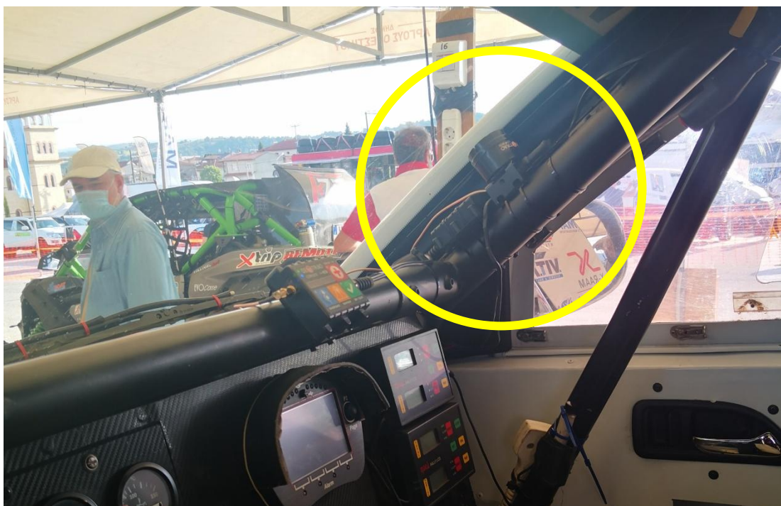
Installation of the Buzzer with bracket on the Roll cage using cable ties.
