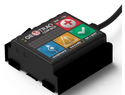
Com-Box unit installed in bracket
